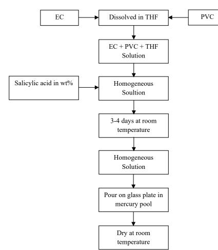
Fig. 2.1 : Flowchart of Preparation of EC-PVC Polyblend thin films
